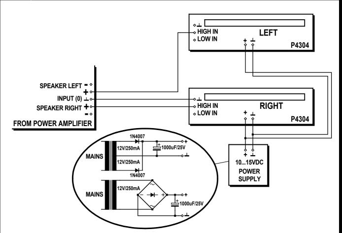
Connect the unit to a suitable supply voltage between 10VDC and 15VDC, this can also be a standard DC adapter. You can also build your own power supply, see diagram. Use a 2x12V transformer, two rectifier diodes and a electrolytic capacitor or use a single 12V transformer with a bridge rectifier and a electrolytic capacitor.
