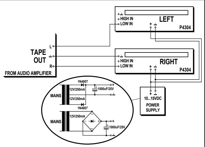
Connect the unit to a suitable supply voltage between 10VDC and 15VDC, this can also be a standard DC adapter. You can also build your own power supply, see diagram. Use a 2x12V transformer, two rectifier diodes and a electrolytic capacitor or use a single 12V transformer with a bridge rectifier and a electrolytic capacitor.
