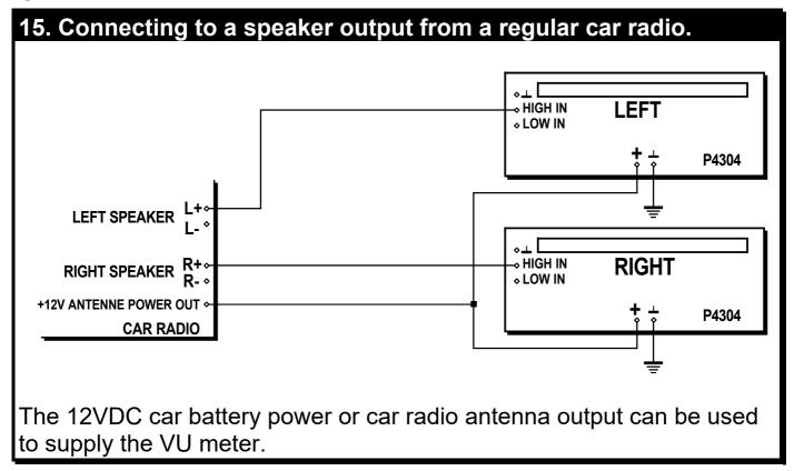
REMARK: Do not connect the unit to a high power car booster or car stereo, this equipment uses isolated ground connection. The connection to this kind of amplifier can cause permanent damage to the amplifier or car radio!
