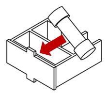
**Step 5:** Rotate fuse holder 180 degrees, insert the fuse holder while the small arrow at 220 – 240 points downward and matches the arrow on the IEC socket. The amplifier is now set for 230V operation.
