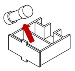
**Step 4:** Insert EU fuse (supplied in the white envelope) into the fuse holder.
