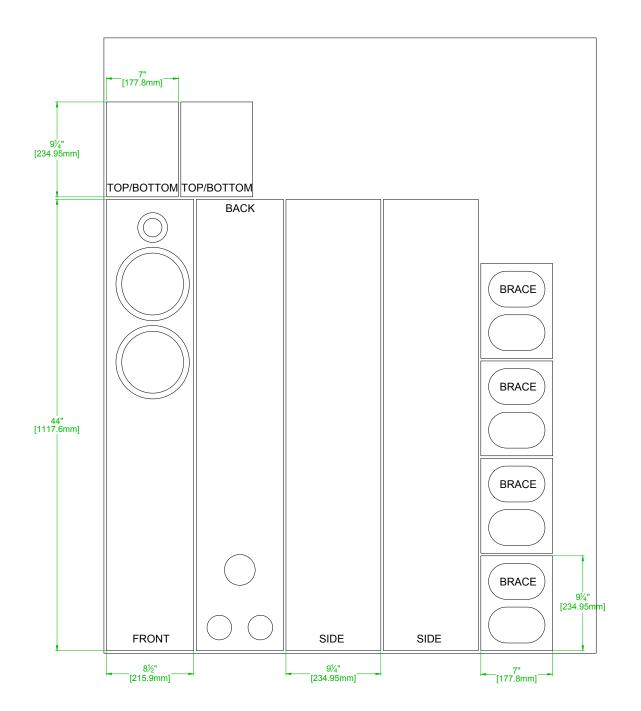
CRITON 2TD-X TOWER SUGGESTED CUT X2 5' X 4' 17-SEPTEMBER-2021 DESIGNED BY D POINSETT/K ARMES | DRAWN BY MM © 2017-18 CREATIVE SOUND SOLUTIONS, LCC
