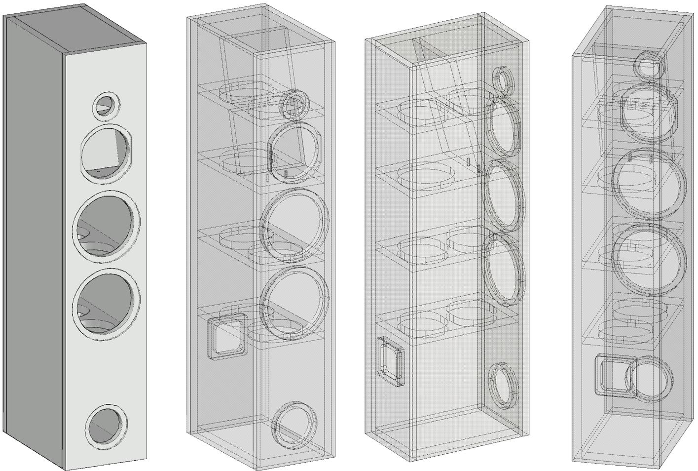
CSS CRITON 3TD-X TOWER IS A 3-WAY TMWW UTILIZING ULTRA LOW DISTORTION DRIVERS IN A PORTED CABINET
