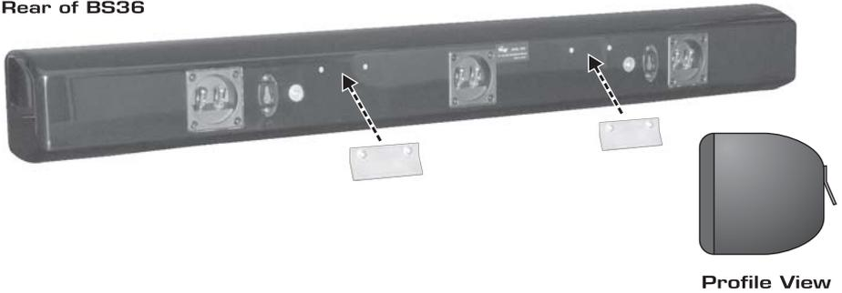
**Step 2:** Identify mounting location and attach wall bracket to the wall using supplied drywall screws. **Do not use nails.** Attach one end first then pivot until bubble is level. Mark holes and install remaining screws. When using the supplied "Wall Dog" screws it is not necessary to locate a wall stud.
