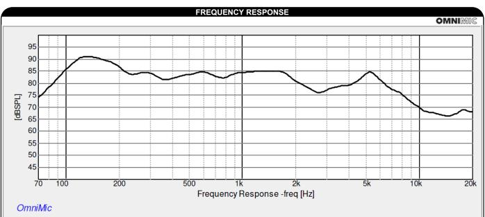
$1/3^{\text{rd}}$  octave smoothing - measurement taken with transducer adhered off-center on a 12" x 12" x 1/2" foam core board in an infinite baffle setup.
