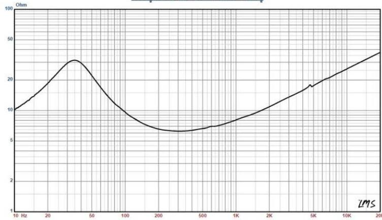
Figure 1: Dayton Audio DSA175 woofer 1 V free-air impedance plot.
