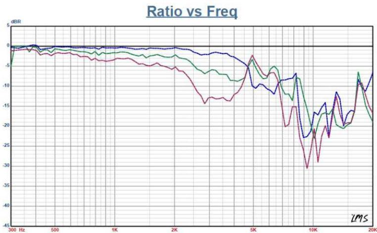
Figure 12: Dayton Audio DSA175 normalized on- and off axis frequency response (black solid = 0°, blue dot = 15°, green dash = 30°, purple dash/dot = 45°).
