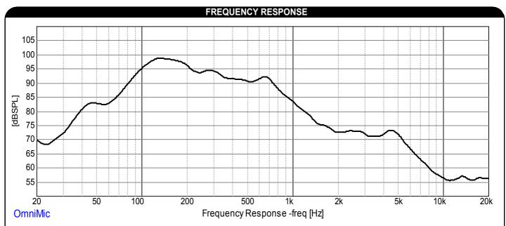
1/3rd octave smoothing - measurement taken with transducer adhered off-center on a 12" x 12" x ½" foam core board in an infinite baffle setup.
