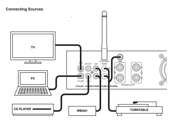
The HTA100 is capable of receiving signals directly from a wide variety of sources. Using high quality cables will ensure the best possible transmission from your connected devices.
