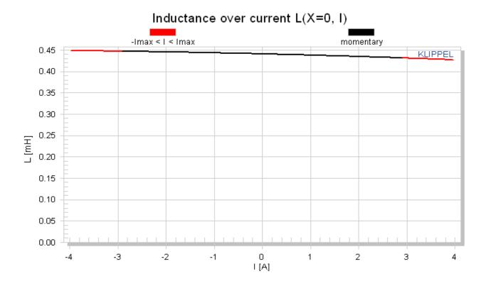
The inductance components Le (x) and Bl(i) of most drivers have a strong asymmetric characteristic. If the voice coil moves towards the back plate the inductance usually increases since the magnetic field generated by the current in the voice coil has a lower magnetic resistance due to the shorter air path.
