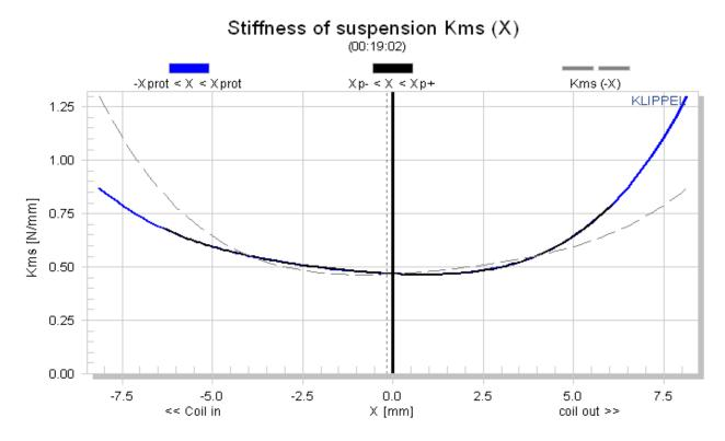
The stiffness KMS(x) describes the mechanical properties of the suspension. It's inverse is the compliance CMS(x)
