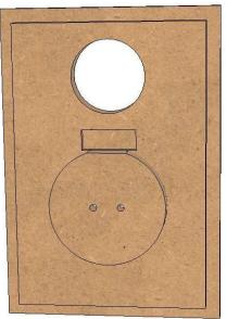
4) With the **Back Panel** (**T**) lying flat, apply a generous amount of glue inside the dado for the brace. Then set the **Brace** (**V**) in place applying enough pressure to fully seat the brace in the dado and ensure glue is spread through the joint (some glue squeeze-out can be expected).
