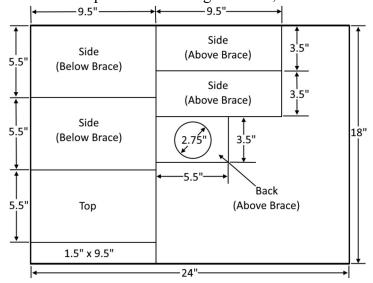
21) Line the top, back (only the port area for now) and sides of the enclosure with the pieces cut on step # 19. Remove the backing from each panel and carefully insert through the driver cutouts. Carefully set the panel into place and press firmly to adhere to the enclosure.
