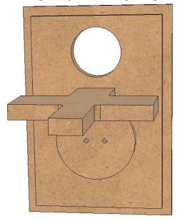
5) Next, glue all mating surfaces of the Back Panel, Brace, and **Side 1 Panel** (**S**). Be sure to apply a generous amount of glue inside the dado for the brace. Then set in place applying enough pressure to ensure glue is spread through each joint and the brace is fully seated in the dado (some glue squeeze-out can be expected).
