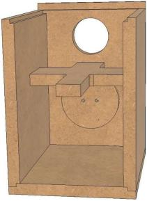
8) Glue all mating surfaces of the Back panel, Side panels, and **Top Panel** (Y). Then set the Top panel in place applying enough pressure to ensure glue is spread through each joint (some glue squeeze-out can be expected)
