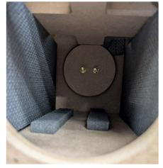
23) Insert the crossover board through the woofer cutout and place it on the bottom of the enclosure towards the back. Place four #8 x 3/4" Pan Head Deep Thread Black Screws (Q) through the four screw holes in the corners of the crossover board. Tighten screws just until the foam standoffs are compressed to about 1/4" – 1/8". Use care when tightening the screws to avoid cracking the crossover board.
