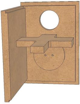
6) Glue all mating surfaces of the Back panel, Brace, and Side 2 Panel (X). Be sure to apply a generous amount of glue inside the dado for the brace. Then set in place applying enough pressure to ensure glue is spread through each joint and the brace is fully seated in the dado (some glue squeeze-out can be expected).
