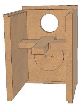
7) Glue all mating surfaces of the Back panel, Side panels, and **Bottom Panel** (**Z**). Then set the Bottom panel in place applying enough pressure to ensure glue is spread through each joint (some glue squeeze-out can be expected).
