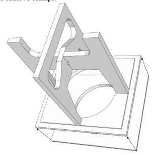
5) This completes the assembly of the included components. The sides and the back of the enclosure need to be cut to the following dimensions using 3/4" thick material (MDF is recommended) before continuing to the next step:
