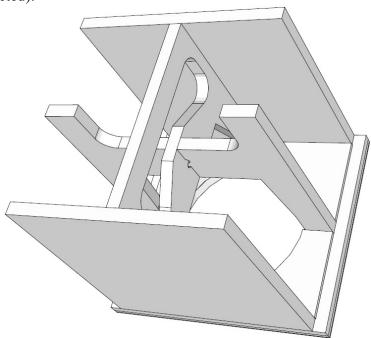
7) Glue all mating surfaces of two remaining side pieces and the baffle/brace assembly then assemble as shown. Make sure that the sides are centered on the baffle/brace assembly. Apply enough pressure to ensure glue is spread through each joint (some glue squeeze-out can be expected)
