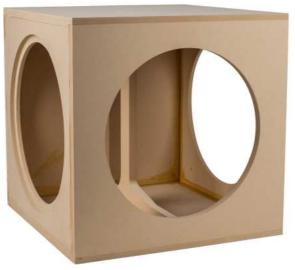
5) Finally, apply a thin layer of glue to the front panel of the enclosure and set the front baffle in place. While ensuring all edges are even and square, position clamps to apply even pressure to the baffle. Using a damp rag or paper towel, wipe away any glue
