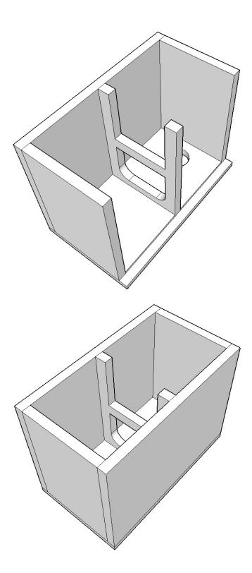
4) Make sure all mating surfaces are flush with each other and clamp glued joints together. Using a damp rag or paper towel, wipe away any glue squeeze-out on the outside of the enclosure (excess glue on the inside is fine). Allow to dry according to the glue manufacturer's recommendations and remove clamps.
