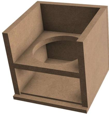
8) Apply a small bead of glue to the inside of all joining surfaces of the other **Top/Bottom Panel (E)** and the enclosure assembly. Then set in place applying enough pressure to ensure glue is spread through each joint (some glue squeeze-out can be expected).
