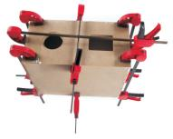
3. Once the glue is dry, remove the clamps. Sandpaper the panels smooth before you finish them. Apply a thin layer of glue to wood veneer and paste it on the enclosure. Press hard and evenly to make sure the veneer is flat and smooth. A piece of wrung hot wet cloth is recommended here to help make the veneer soft enough to be pasted evenly.
