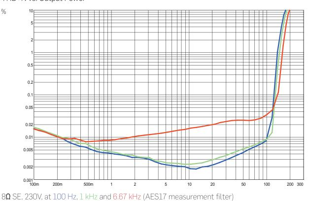
ICEpower 250ASX2 THD+N vs. Output Power W
