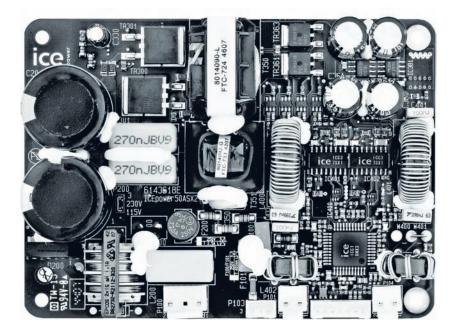
The ASX2 Series is the first ICEpower standard series to adapt our third generation HCOM/MECC SE amplifier topology. The dual amplifier stage is implemented utilizing the ICEpower ASIC chipset.
