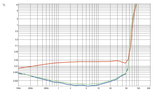
$8\Omega$  SE, 230V, at 100 Hz, 1 kHz and 6.67 kHz (AES17 measurement filter)
