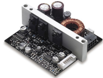
Figure 1: ICEpower250A Size: 8 x 8 x 2.7cm
