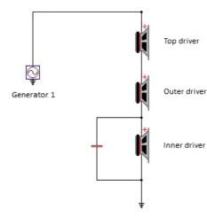
Optional low pass for inner driver 33uF bipolar electrolytic [adjust value as desired]
