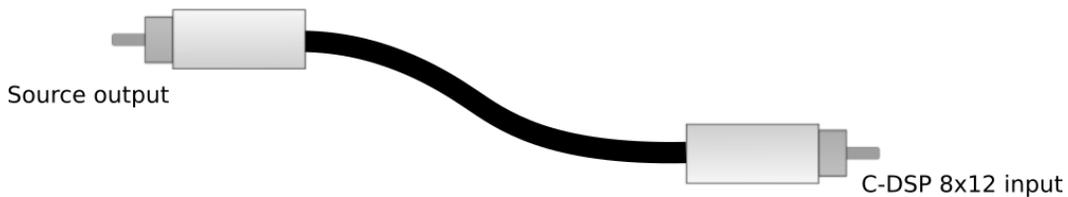
Figure 1. Single-ended RCA connection
