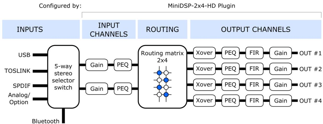
Figure 4. Signal flow in the miniDSP-2x4-HD plugin (simplified)
