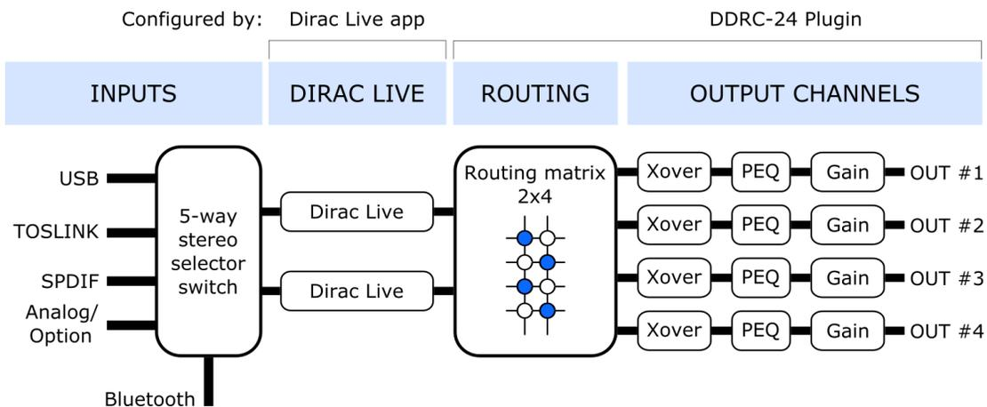
Figure 5. Signal flow in the DDRC-24 plugin (simplified)
