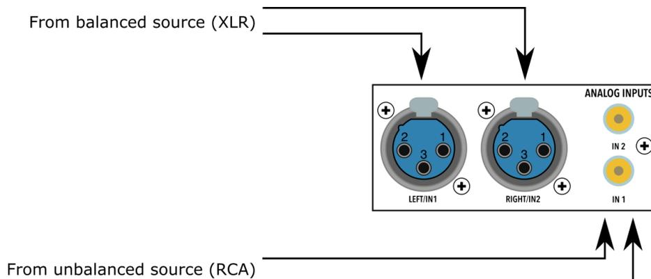
To play from either analog input, use the front panel knob or remote control to select **RCA** or **XLR**.
