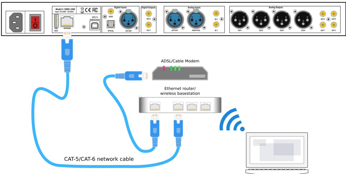
A short Ethernet cable is provided with the unit. If a longer cable is required, these are readily available from computer stores and online. The recommended maximum length of Ethernet cables is 100 meters (330 feet).
