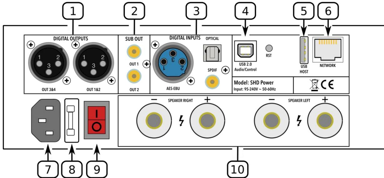
1. **Digital outputs.** Connect downstream digital equipment with AES-EBU cables. These outputs each carry a stereo signal. The data format is 24-bit 96 kHz. Connected equipment must therefore be able to accept a 24-bit 96 kHz input signal.
