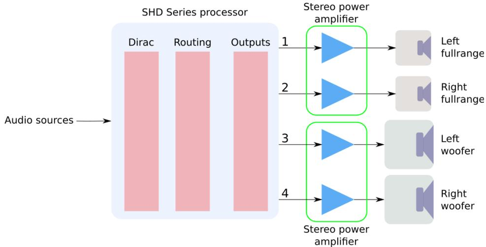
In this type of configuration, use crossover filters to split the frequency range to the woofers and main speakers. The crossover frequency may range from 80 Hz for true subwoofers up to perhaps 300 Hz for smaller woofers.
