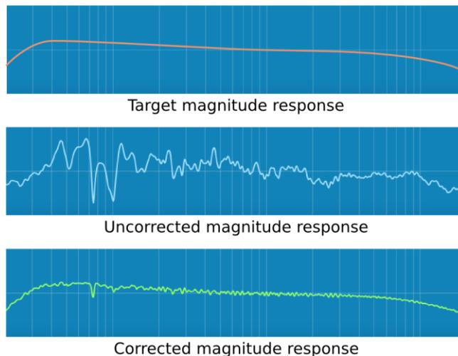
In addition to correcting magnitude response, Dirac Live® corrects the system's *impulse response*, which reflects how the system responds to a sharp transient such as a drumbeat. Reflections, diffraction, resonances, misaligned drivers, and so on, all combine to smear out the transient. Correcting the impulse response makes the speaker in the room behave much more like an ideal loudspeaker. The impulse response is a critical factor for accurate sound-staging, clarity and bass reproduction.
