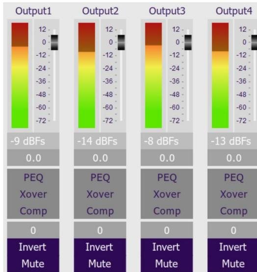
Each channel has an individual gain adjustment slider and a graphical and numerical display of the current signal level on that channel. A comprehensive set of signal processing functions is accessed with the buttons PEQ (parametric EQ), Xover (crossover) and Comp (compressor/limiter). Each channel also has individual time delay, invert, and mute.
