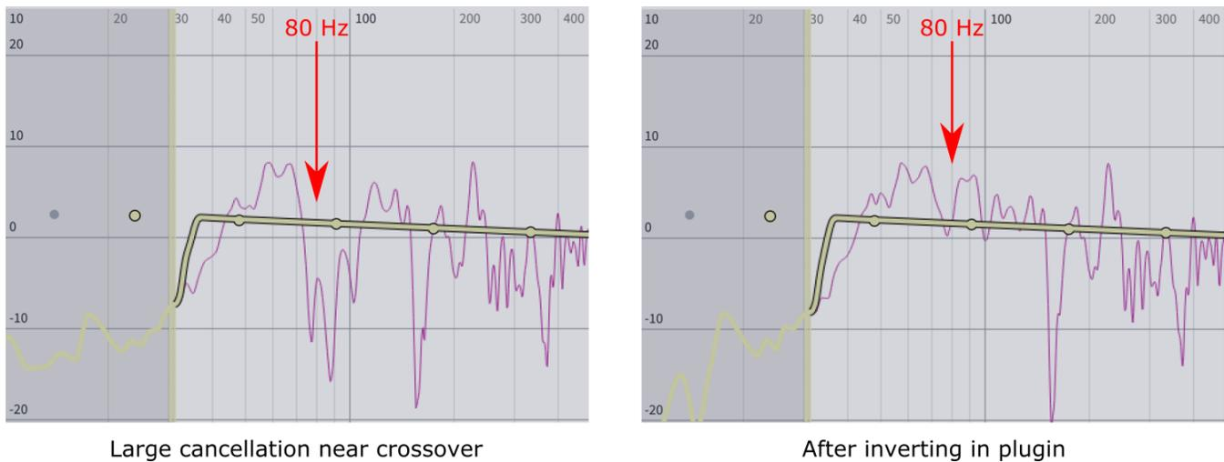
Figure 5. Example showing effect of subwoofer inversion
