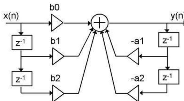
A single biquad like this can perform a great many functions, including all of the functions of a single parametric EQ filter, one 6 or 12 dB/octave high pass or low pass crossover filter, and more. Biquads are combined in series (cascaded) to create more complex filters. The function that each biquad performs is determined by just five numbers:  $b_0$ ,  $b_1$ ,  $b_2$ ,  $a_1$ , and  $a_2$ . These numbers are called the *coefficients*.
