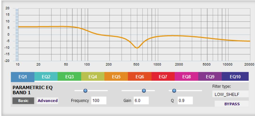
There are ten parametric EQ filters on each output channel. The window displays a frequency response graph showing the combined response of all enabled parametric filters on that channel. For example, the response curve above has a low-shelf boost at 100 Hz, a dip at 500 Hz, and a high-shelf cut at 5000 Hz.
