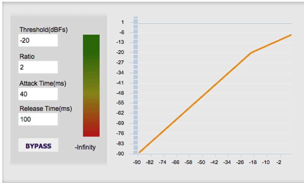
(Note that the compressor algorithm is bypassed by default, so click on the **Bypass** button to see the curve as shown here.)
