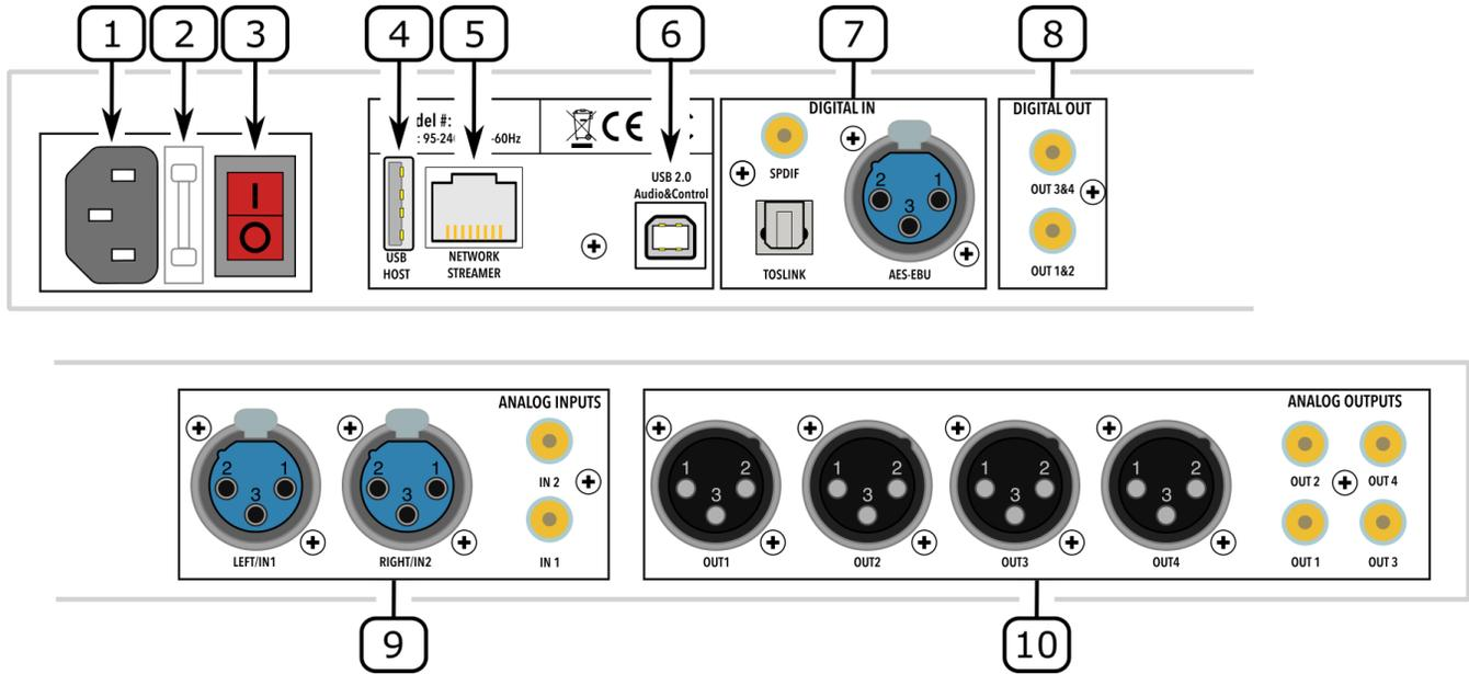
1. **Power inlet.** Connect a standard IEC C13 cable here. The mains supply voltage can be in the range 95 to 240 VAC, 50 to 60 Hz.
