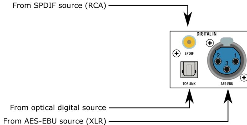
To play from any of these sources, use the front panel knob or remote control to select **AES-EBU**, **SPDIF**, or **TOSLINK**.
