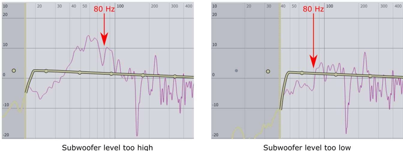
Figure 4. Examples of subwoofer level imbalance
