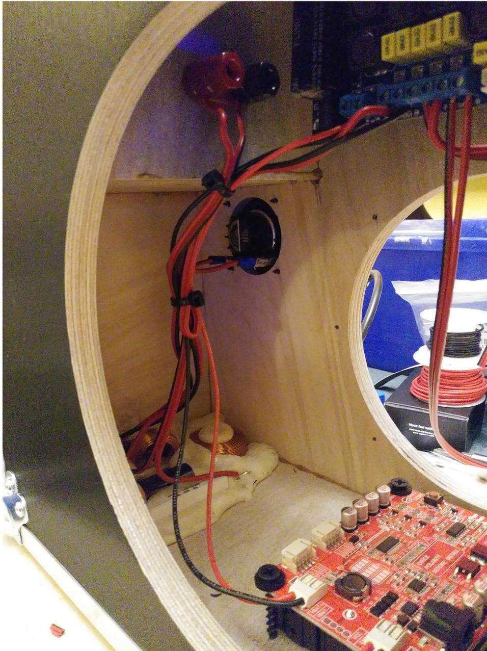
**33)** Connect stripped ends of the red/black speaker wire from the amplifier's **BASS** output to the corresponding spring loaded terminals on the Dayton Audio DCS165-4 6-1/2" Classic Subwoofer. Place driver in opening and secure in place using 8 x #8 x 3/4" Deep Thread Pan Head Screws being careful not to strip out the holes (a power drill is not recommended).
