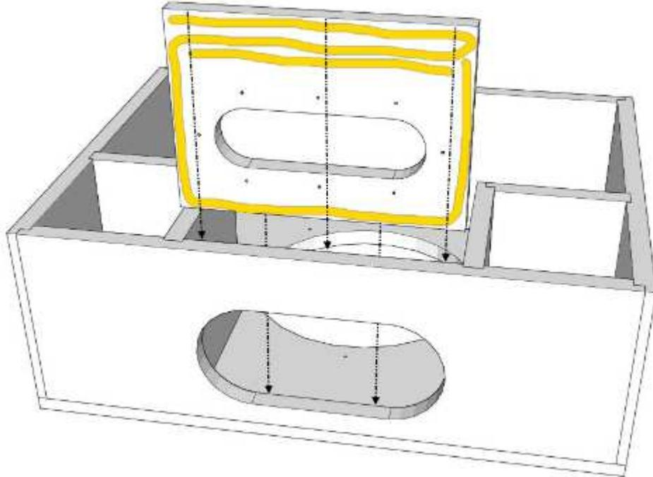
8) Apply a small bead of glue to the inside of all the rabbeted edges and dadoes on the front panel. Then set in place on the rest of the enclosure, due to the tight fit a firm tap may be needed. Apply enough pressure to ensure glue is spread through each joint (some glue squeeze-out can be expected).
