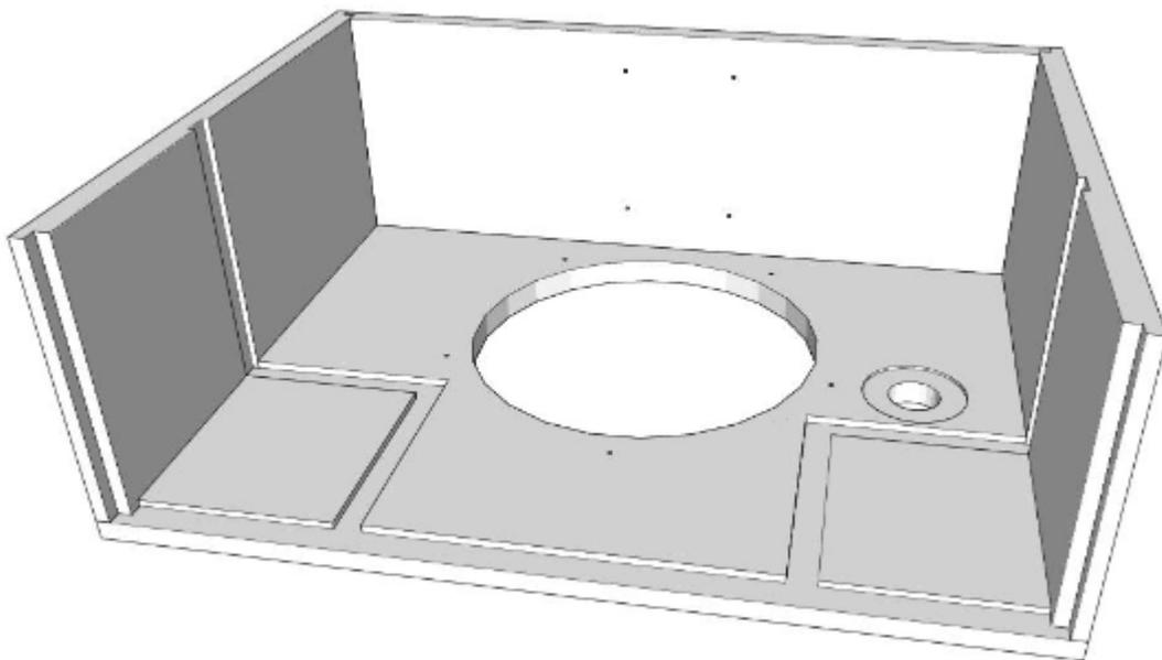
5) Apply a small bead of glue to the inside of the rabbeted edges and dadoes of all joining surfaces of the horizontal inner baffles, vertical inner baffles, back, and side panels. Then set in place applying enough pressure to ensure glue is spread through each joint (some glue squeeze-out can be expected).
