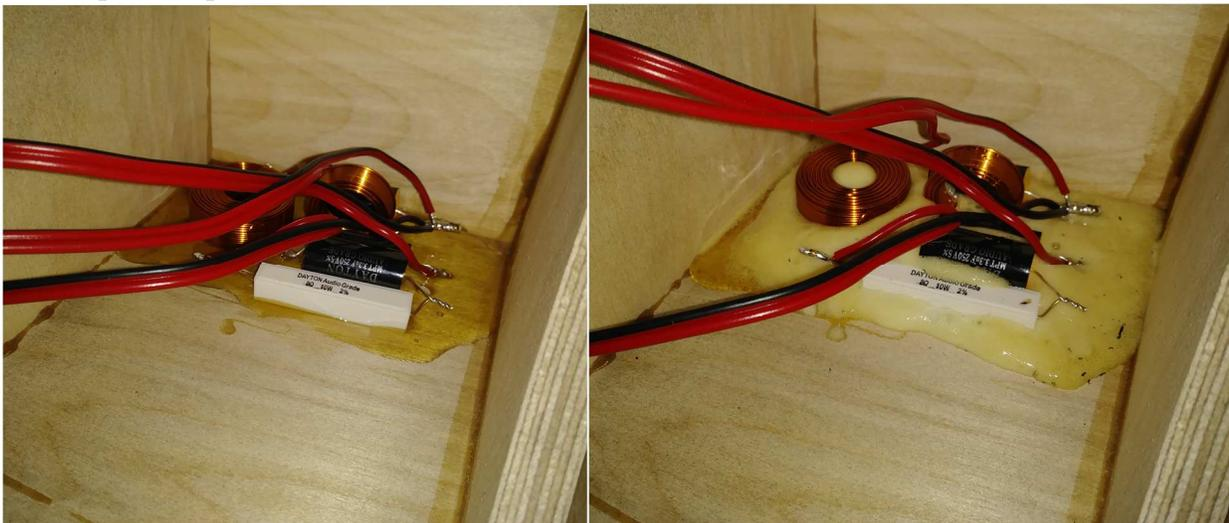
17) Cut 2 6" pieces of red/black speaker wire and strip 1/4" - 1/2" of insulation from each end. Then crimp 2 x #8 blue ring terminals to one end of each wire and 2 x 0.205" blue female disconnects to the other end of each wire.
