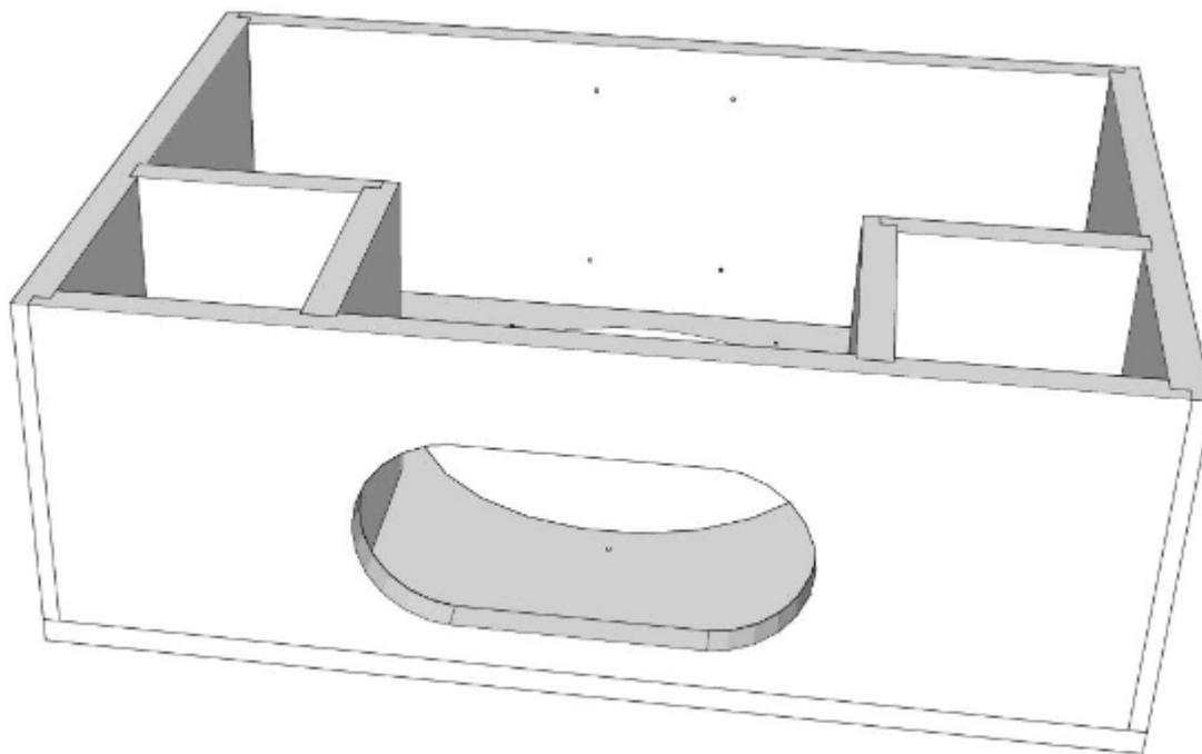
7) Apply a small bead of glue to the front of the amp mounting panel. Keep at least 1-1/4" away from the oval shaped opening, as shown. Also apply a small bead to each outside edge of the amp mounting panel. Then set in place as shown, applying enough pressure to ensure glue is spread through each joint (some glue squeeze-out can be expected).
