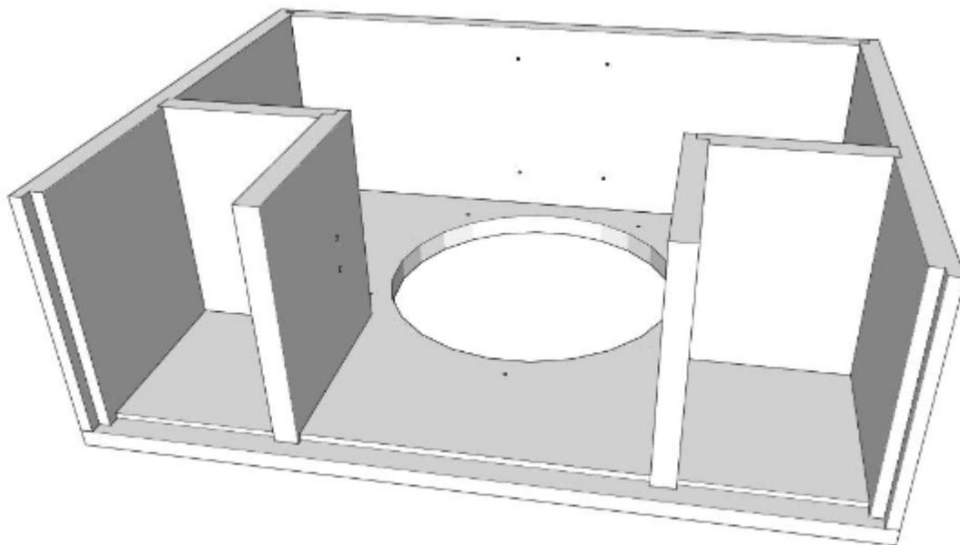
6) Apply a small bead of glue to the inside of the rabbeted edges and dadoes of all joining surfaces of the top, vertical inner baffles, back, and side panels. Then set in place applying enough pressure to ensure glue is spread through each joint (some glue squeeze-out can be expected).
