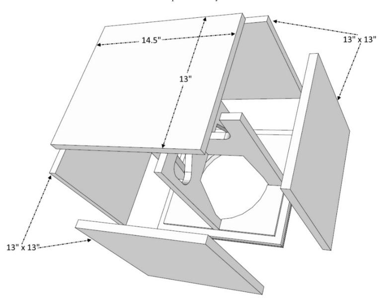
6) Glue all mating surfaces of two opposite side pieces and the baffle/brace assembly then assemble as shown. Make sure that the sides are centered on the baffle/brace assembly. Apply enough pressure to ensure glue is spread through each joint (some glue squeezeout can be expected).
