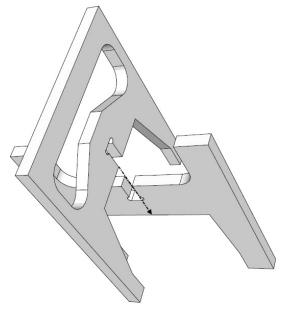
3) Glue all mating surfaces of the brace assembly and primary baffle then assemble as shown. Make sure that the brace assembly is centered on the primary baffle. Apply enough pressure to ensure glue is spread through each joint (some glue squeeze-out can be expected).
