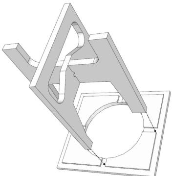
4) Evenly spread a thin layer of glue to the back side of the secondary baffle and assemble as shown. Make sure that the secondary baffle is centered on the primary baffle. Clamp baffle and brace assembly together so that even pressure is applied to all glued surfaces. Using a damp rag or paper towel, wipe away any glue squeeze-out from between the baffles and inside the rabbeted edges. Allow to dry according to the glue manufacturer's recommendations and remove clamps.
