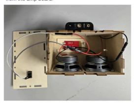
Step 10. Make sure all the slots in the wood panels are installed all the way into the matching wood panels. Use the 14 M3 x 10mm screws to secure the wood panels together. Five screws on the top and on the bottom, and two screws for the front and back panel.
