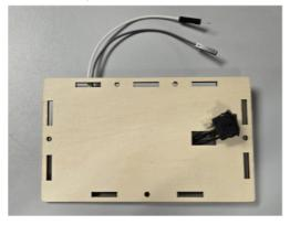
**Step 9.** Plug the white and gray wires from the switch into the red wire from the battery holder and the amp board. Plug the black wire from the battery holder into the loose black wire from the amp board.
