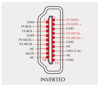
Note: This option is used to match different I<sup>2</sup>S interface standards, please check the interface definition of the signal source before use
