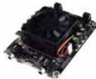
2 x 100Watt Class D Audio Amplifier Board - TDA7498 (AA-AB32189)
