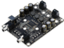
2 x 30 Watt Class D Audio Amplifier Board - TPA3118 (AA-AB32472)
