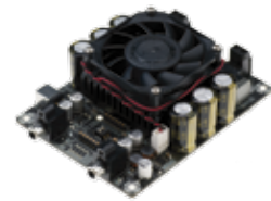
2 x 200Watt Class D Audio Amplifier Board - T-AMP(AA-AB32281)
