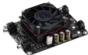
2 x 160Watt Class D Audio Amplifier Board - TDA7498E (AA-AB32361)
