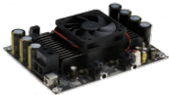
2 x 150Watt Class D Audio Amplifier Board - TAS5613 (AA-AB32221)
