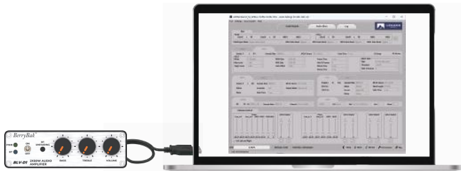
Figure 1: Connect the BLV-D1 to a personal computer or laptop and ensure that you have installed the ACP Workbench application.
