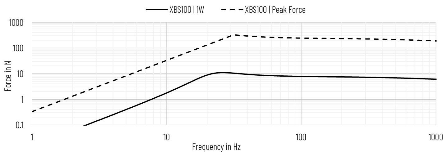
Note: Peak force is estimated from long-term maximum input power and the mechanical Xmax, assuming a linear model.
